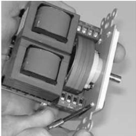
1.) Remove the control knob by pulling it away from the volume control post. Then, use a small screwdriver or other similar tool to gently push the plastic tabs through the metal back plate.
