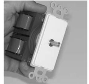
5.) Gently (but firmly) press the new plastic faceplate onto the metal back plate. Then, place the new control knob onto the volume control post.
