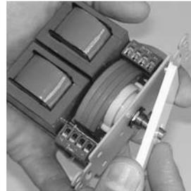
4.) Align the desired trim color faceplate tabs in the top two holes in the metal back plate. Then, make sure the other two plastic tabs align with the other two holes in the metal back plate.
