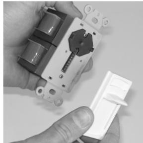
6.) Set the volume control's level to maximum and move the slide knob to the top of the faceplate.
