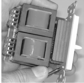
1.) Use a small screwdriver or other similar tool to gently push the plastic tabs through the metal back plate.
