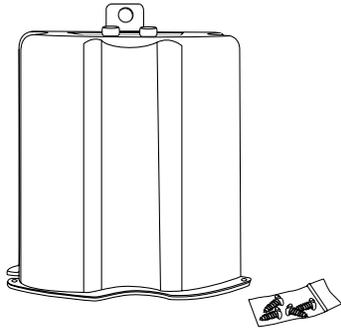
**NOTE:** Carefully tuck the speaker wires inside back can so they do not get pinched.
