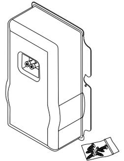
**NOTE:** Carefully tuck the speaker wires inside back can so they do not get pinched.
